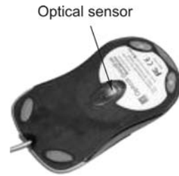
Fig. 4.3 The lower portion of the optical mouse
