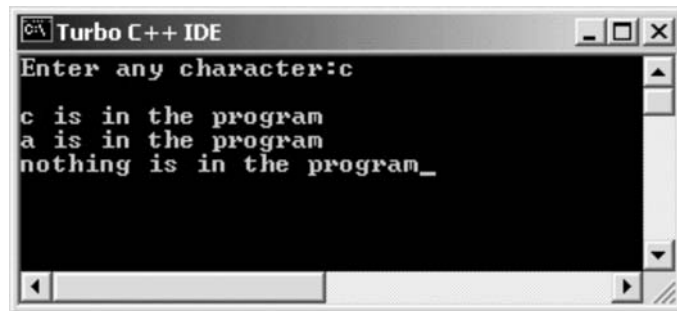
Fig. 16.13 Explaining the usage of switch case statement without break
